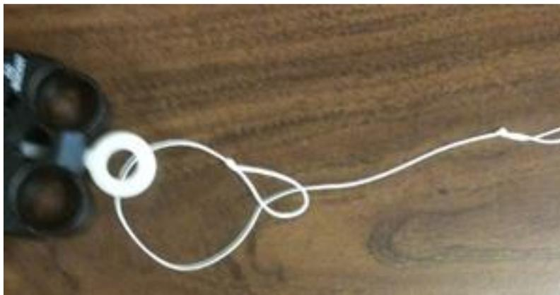
For Part G, you must connect the string to two Force Sensors. To do this, unscrew the plastic connectors from the sensors, connect them with two loops in the strings, then screw the connectors back into the sensors.
