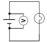
Instructions on how to use a multimeter as a voltmeter are given in Appendix 2.B. Use a multimeter to measure the voltage of the battery. The rated voltage is written on the front of the battery. How do the two values compare?
