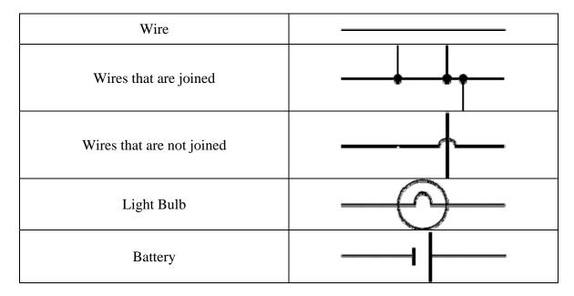
For the Battery, the positive terminal is on the right and the negative terminal is on the left. Here is a mnemonic for remembering this: a + symbol has more line in it than –, and the longer line of the battery is the + terminal.
