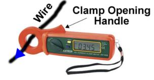
When the current is flowing in the direction shown, the reading will be positive; if the current is flowing in the opposite direction to that shown the reading will be negative. There is a small arrow on the inside of the jaws of the clamp indicating the current direction shown in the figure.
