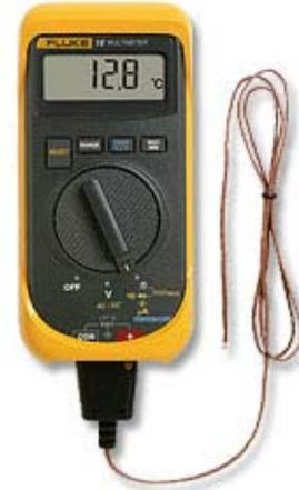
Finally, then we would write the temperature as  $12.80 \pm 0.05$  °C.
