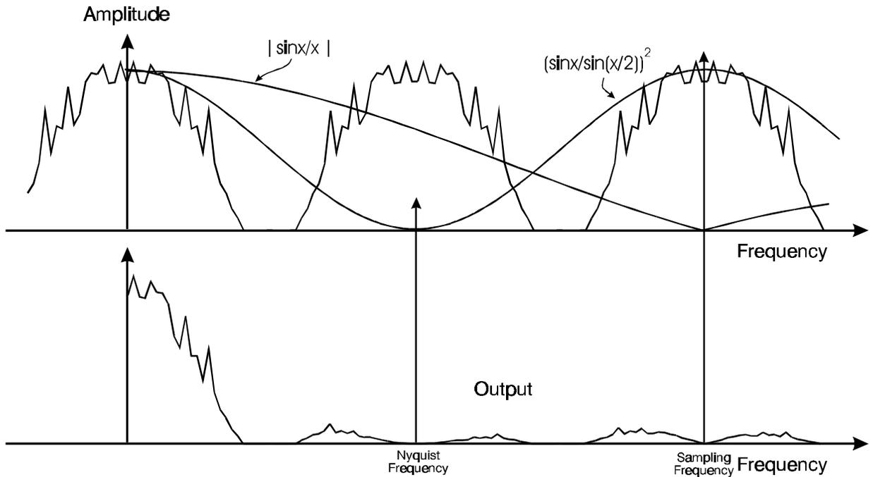
Interpolation Filter compared with "Hold" filter
