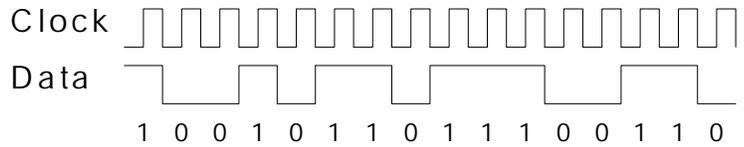
**Separate Clock Synchronous Data**
