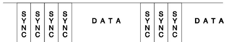
**Synchronous Transmission in Blocks With "Sync"**
