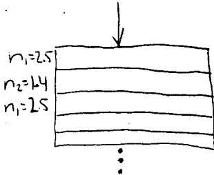
$$R = |r|^2 = \left( \frac{n_1 - n_2}{n_1 + n_2} \right)^2 \quad \text{in which the light passes from medium with ref. index } n_1 \text{ to that with ref. index } n_2$$
