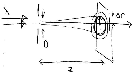
If the light is collected by a lens, then  $z \approx f$  (since light is incoming from  $\infty$ ),  $\Delta r = \frac{1.22\lambda f}{D}$  ~~for diffraction~~
