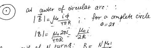
for a cost of N turns:  $B = N \frac{M_0 I}{2R}$ For two concentric circles at their centre  $\vec{B} = \vec{B_i} + \vec{B_o} = |B_i| |B_0| = M_0 \left(\frac{i \cdot N_i}{R_i} - \frac{i \cdot N_i}{R_0}\right) = 0$   $\vec{i}_0 = \frac{i \cdot N_i R_0}{R_i \cdot N_0} = \frac{GA \times 120 \times 0.017}{D.0/2m \times 15D} = \frac{G.84}{0.02m \times 15D}$
