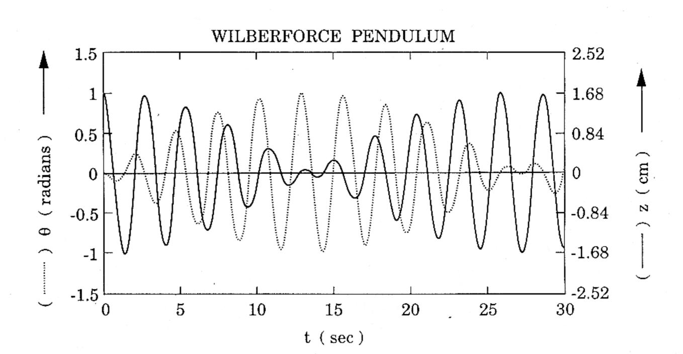
Fig. 2. Coordinates z and  $\theta$  as a function of time for our Wilberforce pendulum, when the pendulum is started in the longitudinal mode by lifting the bob straight up and releasing it from rest.
