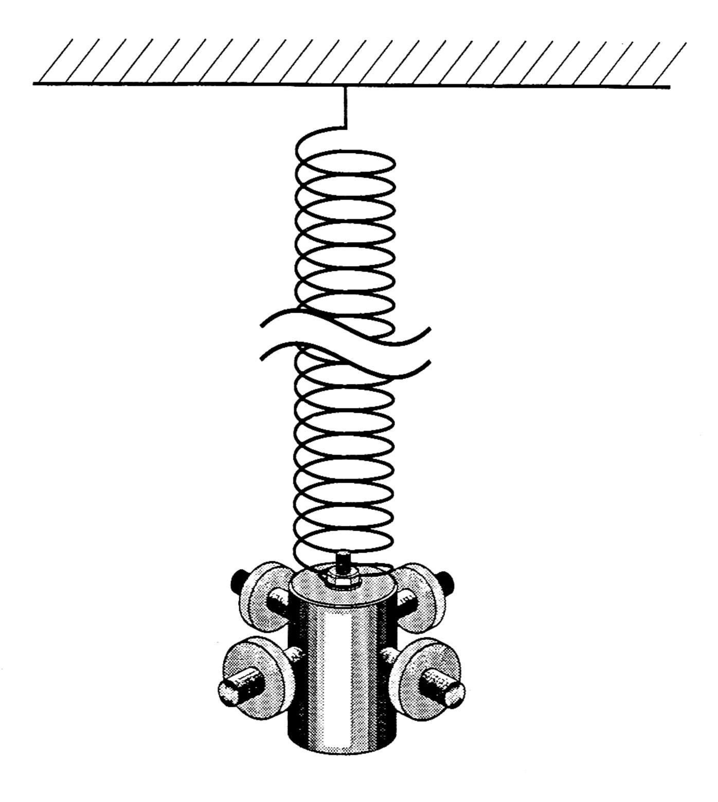
Fig. 1. Sketch of our Wilberforce pendulum. The actual length of the spring is almost 2 m.
