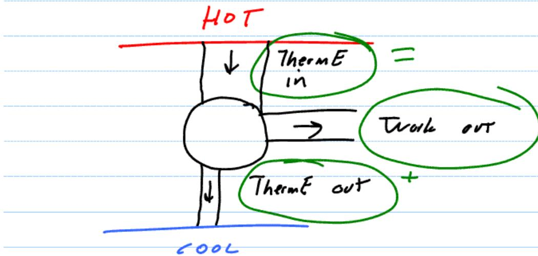
$$\text{efficiency} = \frac{\text{Work out}}{\text{ThermE in}}$$
