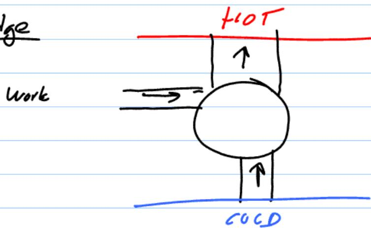
No heat engine can be 100% efficient
