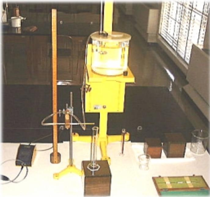
The coefficient of viscosity of a fluid can be found from measurements of the volume rate of flow through small tubes. For simple analysis to be possible laminar or *streamlined* flow must prevail. Conditions of flow can be described by a dimensionless quantity, Reynolds Number,  $N_R$ .  $N_R$  is defined as:
