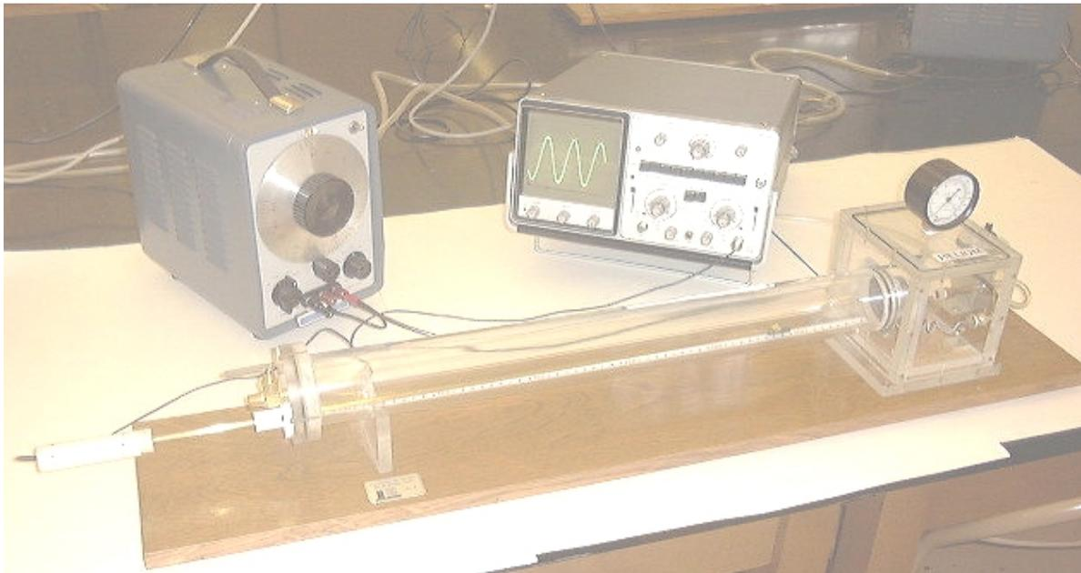
This experiment is very similar to the *Standing Waves* experiment, except that this is performed in a pure gas (Nitrogen). Consequently an accurate value of the constant  $\gamma$  can be determined.
