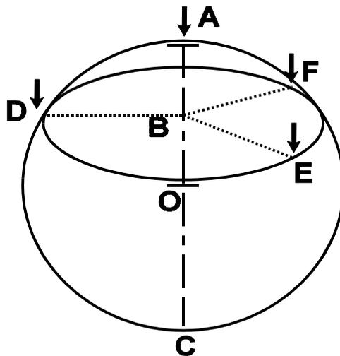
Measure  $d$  with vernier calipers. To do this bring the central foot down to the position on the level with the others, press the spherometer lightly on the page of your notebook and measure the distance between the pricks. Record the three distances and take the mean.
