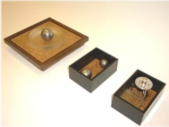
On first glance the motions of a sphere on a concave spherical surface of radius of curvature  $R$  might appear to be that of a simple pendulum of length  $R$ . However, a quick recognition of the effects of the moment of inertia of the sphere leads to a different conclusion. If a sphere of radius  $a$  undergoes small oscillations on a surface of radius  $R$ , without slipping, the period is given by:
