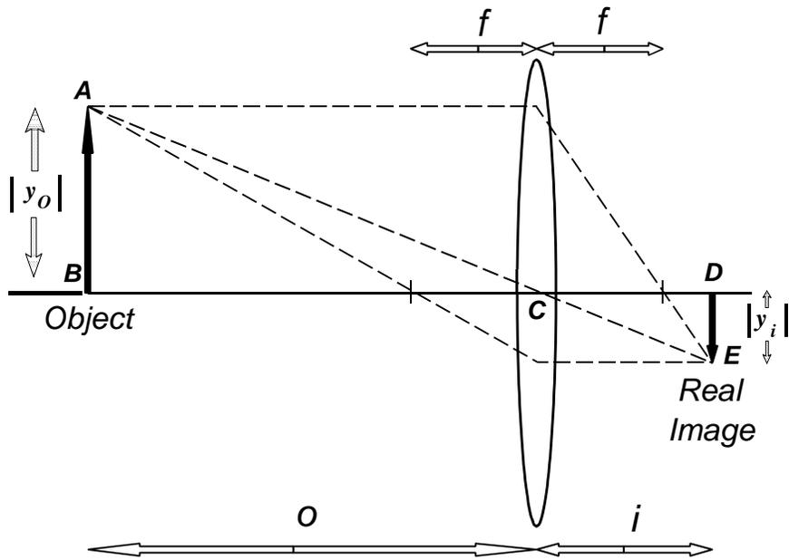
**Figure 2.** - Image formation with a thin lens.
