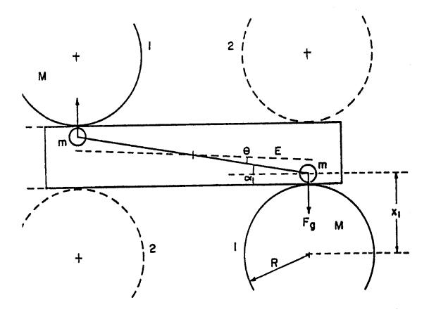
Figure 1. - Top View of Cavandish apparatus
