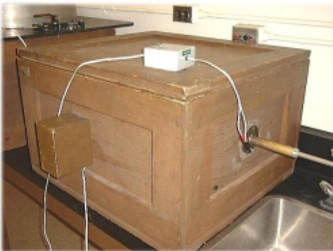
The apparatus is the acoustic analogue of the Michelson optical interferometer. In our case, the beam splitter is a sheet of paper. The source is a “tweeter” (loud speaker) driven by an oscillator; it has a range from  $\sim 3$  kHz to 10 kHz. Each time the movable reflector is displaced through  $\frac{1}{2}\lambda$ , so that the path length changes by  $\lambda$ , the interference in the recombined beam going to the receiver is the same.
