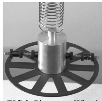
FIG.2: Photogate Wheel attached to the brass cylinder
