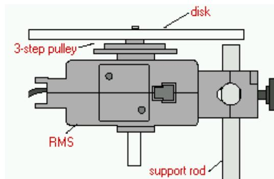
Place a bubble level on the aluminum disk and level the stand so that the bubble stays in the centre as you rotate the disk. This means that the axis of rotation is vertical.
