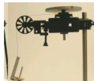
Masses are to be hung from a thread attached to the horizontal three step pulley and this will provide the accelerating torque.
