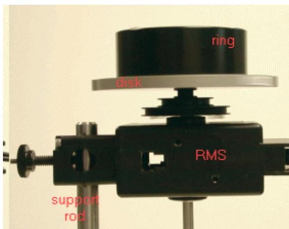
Place a bubble level on the aluminum disk and level the stand so that the bubble stays in the centre as you rotate the disk. This means that the axis of rotation is vertical.
