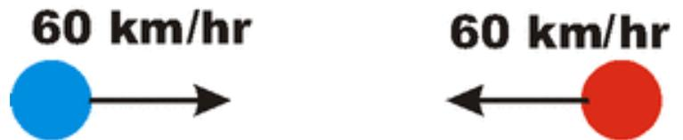
When they two objects collide they stick together. Since before the collision the two objects had equal masses and were moving in opposite directions at the same speeds, their *inertia* or *momenta* were equal and opposite. Thus after the collision they will be stationary relative to us. This is an example of the *Principle of Inertia*, also called *Conservation of Momentum*.
