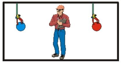
If the room is on a rocket ship that is accelerating upwards at  $9.8 \text{ m/s}^2$  with respect to some inertial frame of reference in free space, then relative to us the balls will fall straight down, accelerating at  $9.8 \text{ m/s}^2$ , until they strike the floor of the room. Thus the distance between the balls remains constant while they are falling.
