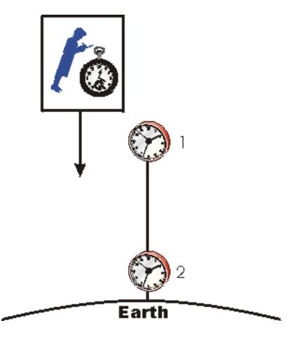
But, since we are in free fall our speed with respect to the Earth and the two Earth-bound clocks is increasing: we are accelerating down at  $9.8 \text{ m/s}^2$  relative to the Earth. So when we pass Clock 2, its speed with respect to us is greater than the speed of Clock 1 when we passed by it.
