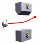
If we take a beam of electrons from an electron gun and run it through the magnet, we see something strange: all electrons are deflected up by some fixed amount or deflected down by exactly the same amount, and which for each individual electron appears to be random. If the deflection is up, we say the electron is "spin up" and if it is deflected down we say it is "spin down."
