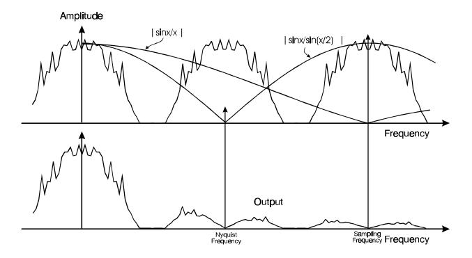
We finally have to account for the fact that the DAC is still going to hold the value between samples which gives a sincx response appropriate to a sampling rate of T/2. If we multiply the two "filters" together we find that the effect of both operations is actually to return the system to the performance of the the original series sampled at 1/T - a long way around to get nowhere!
