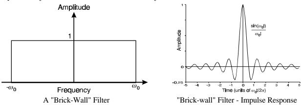
Here's another example. Consider a filter whose passband is so tight that it can be considered to be a delta function in frequency space at frequency  $\omega_0$ . The impulse function of this filter is:
