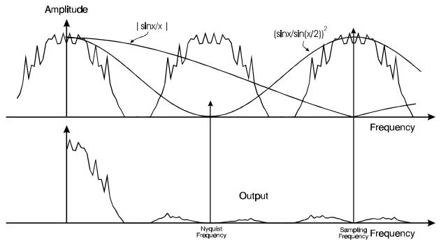
Interpolation Filter compared with "Hold" filter
