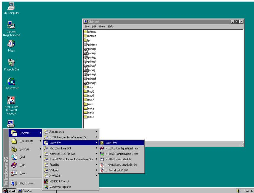
When we use the notation **Start>>Programs>>Labview>>Labview** we are asking you to follow a series of menus starting from the first item which should be visible in the current window. You can see the entire tree for this operation on the screen below.
