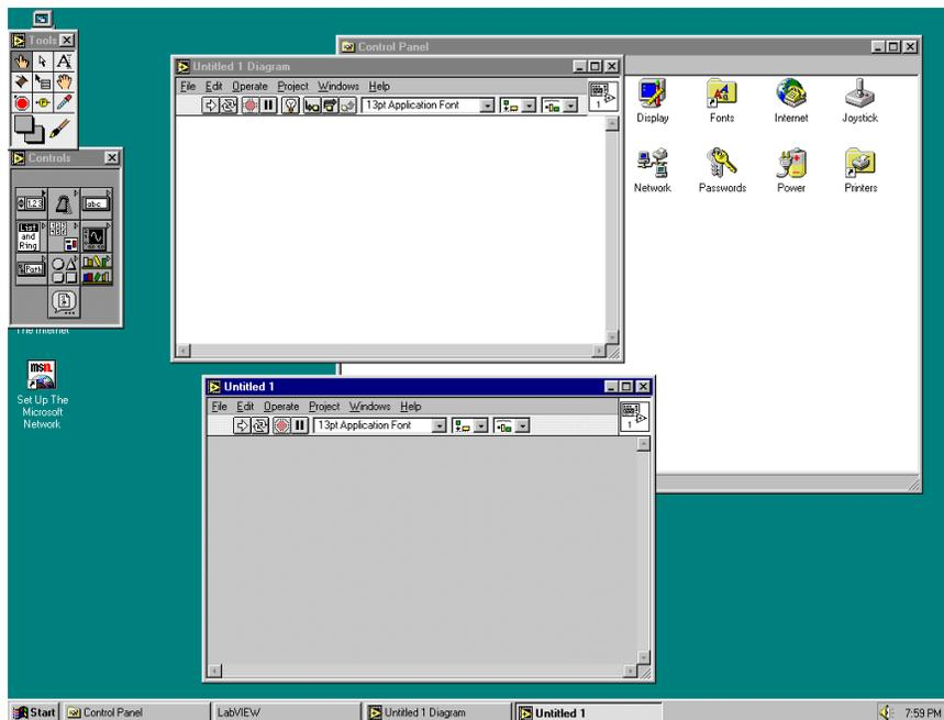
Let's concentrate first on the window with the grey background - the *front panel*. The window is blank (no panel designed yet) with seven icons along the top of the window and a large one in the top right. The seven icons are used to design a front panel and the large one represents the entire front panel when we are making or modifying a sub-VI.
