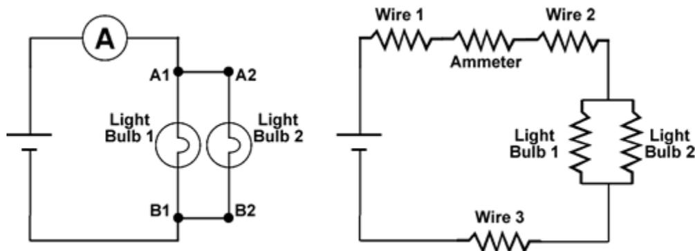
The current in the circuit may be over 1A. As discussed in Appendix 2 of the Electricity and Magnetism Module 2, the inputs to the ammeter should be connected to **10A COM** and **10A** sockets.
