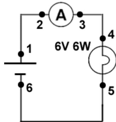
For the light bulb, you will need to know that as it heats up its resistance changes. Thus when doing measurements of a light bulb in a circuit, be sure to give it a few seconds to reach equilibrium.
