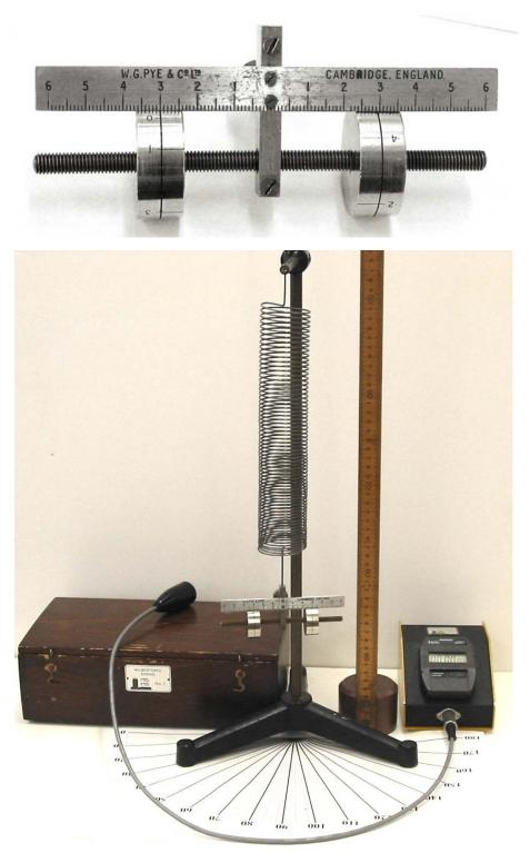
The simple treatment of a mass on the end of a spring that you learn in lectures says that when the mass is oscillating up and down the period should depend only on the particular spring used and the total mass on the end of the spring. The period for this massless spring is not applicable for the Wilberforce Spring: *i.e.*,
