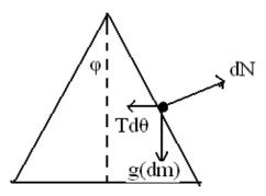
The small piece of chain has three forces acting on it: the normal force, the tension force, and the gravitational force. Hence for equilibrium or horizontal and vertical forces:  $Td\theta - \cos(\varphi)dN = 0$
