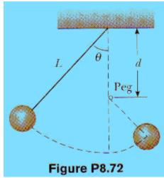
(a) Energy is conserved in the swing of the pendulum, and the stationary peg does no work. So the ball's speed does not change when the string hits or leave the peg, and the ball swings equally high on both sides. (b) The pendulum is started at  $\theta = 90^{\circ}$  and we want it to complete an entire circle about the peg. First we note:
