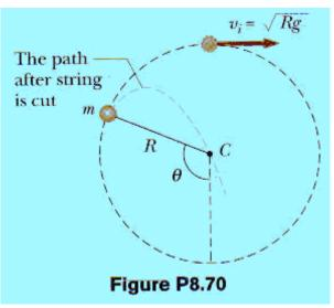
If we define the zero height level to be at the centre of the circle, the angle the string makes with this horizontal is  $\phi = \theta - 90$  degrees. Therefore  $x = R \cos \phi$   $v_x = v_f \sin \phi$
