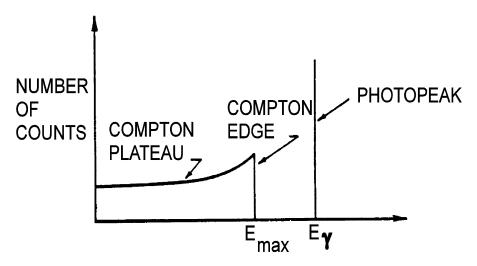
**Figure 2. -** Idealization of gamma-ray spectrum showing photopeak and compton plateau
