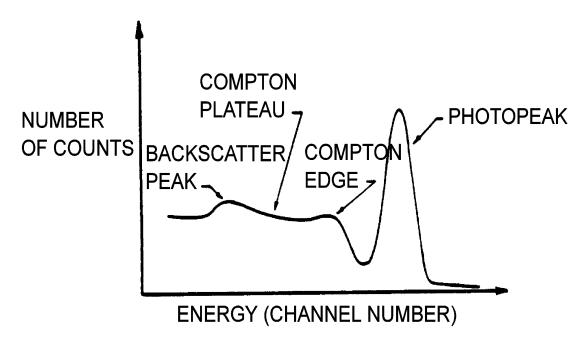
Figure 4. - A Typical Gamma-Ray Spectrum
