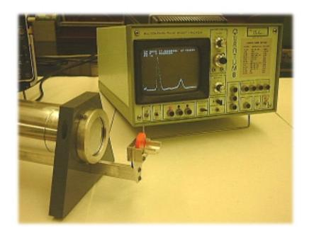
In this experiment you will investigate the properties of gamma-ray spectra observed with scintillation counter (a sodium iodide, NaI(Tl) scintillation counter and a multichannel analyzer). You will calibrate the detection system using radioactive sources (available at the Resource Centre) with gamma-rays of known energy and then you will measure the energy of a gamma-ray from unknown source.
