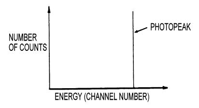
**Figure 1. -** Idealized Picture of Gamma-Ray Spectrum Showing Only the Photopeak
