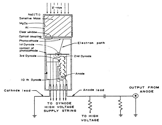
Figure 3. - Sodium Iodide Scintillation Detector
