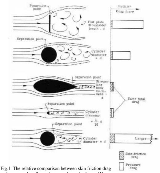
and pressure drag for various aerodynamic shapes [3].
